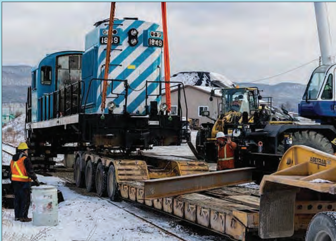
The locomotive's cab and main structure are put on another flat trailer.
